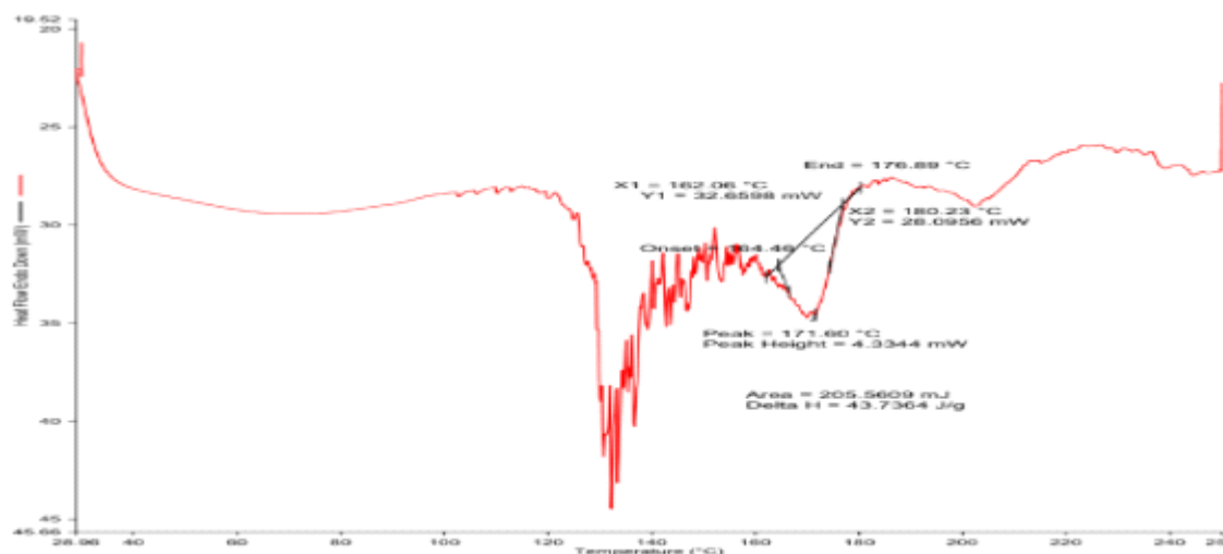
Fig.5- DSC thermogram of CPC F3 showing a broad endothermic peak at 171.60/ °C, confirming complex formation.
